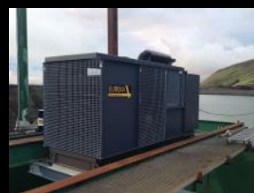
Hydraulic Power Pack
