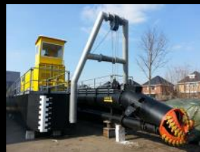
Cutter dredger Delta
